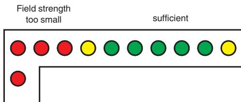
The field strength is sufficient, if LEDs light up within the green area. The field strength should be checked over the entire length of the cylinder. In the area of the piston the field strength should be the highest.
